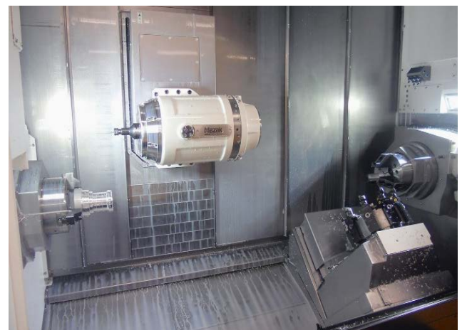
Machine room with turning and milling spindle
