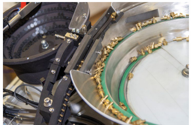
Spiral conveyors area
